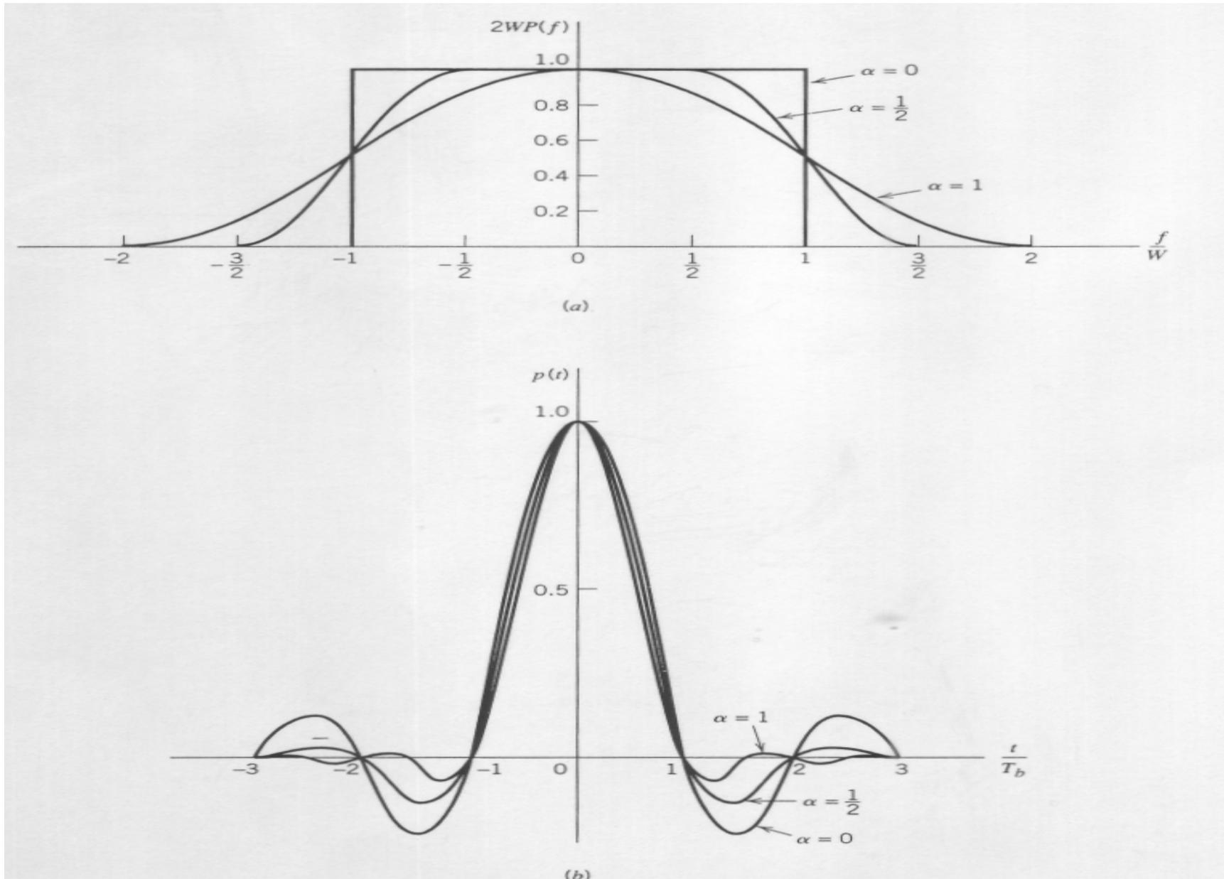
**FIGURE 3-4** Responses for different roll-off factors. (a) Frequency response. (b) Time response.
