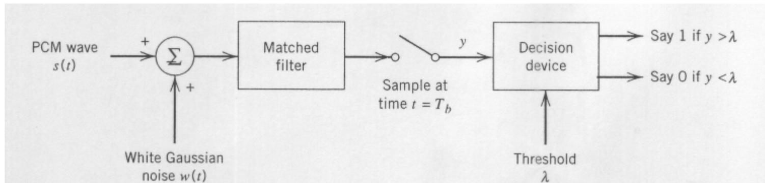
FIGURE 3.3 Receiver for baseband transmission of binary-encoded PCM wave using polar NRZ signaling.
