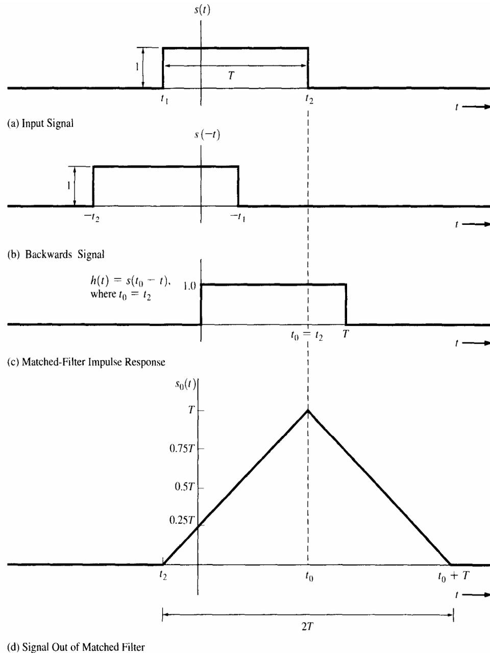
FIGURE 3-2 Waveforms associated with the match filter of Example 3-1
